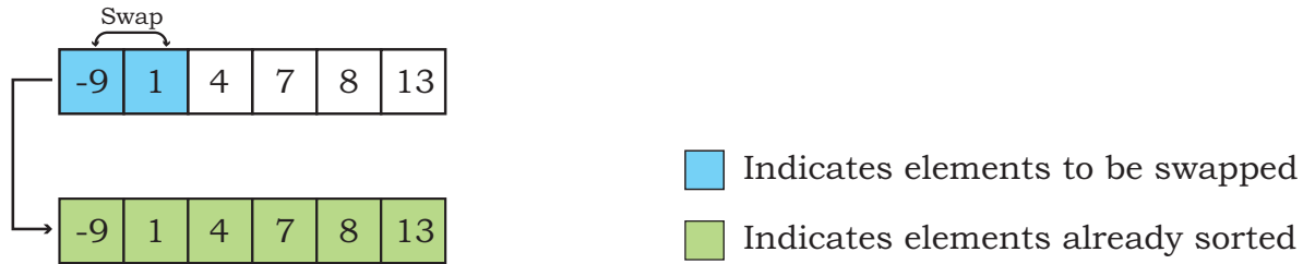
Figure 5.1: Comparisons done in different passes of Bubble sort
