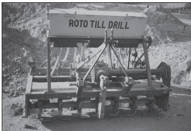
Fig. 3.12 : Roto Till Drill—A modern agricultural equipment
