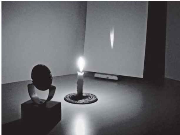
Fig. 15.15 Real images formed by a concave mirror
