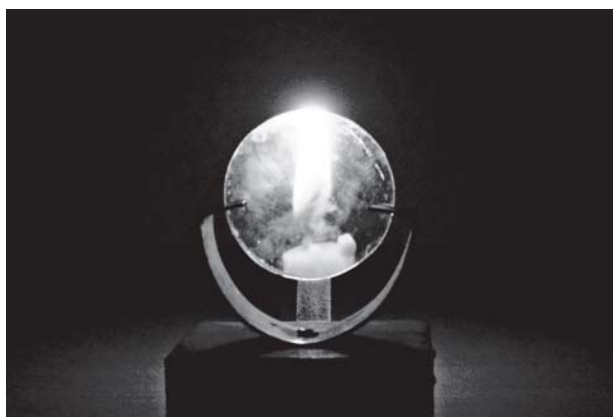
Fig. 15.26 Virtual image formed by the convex lens
