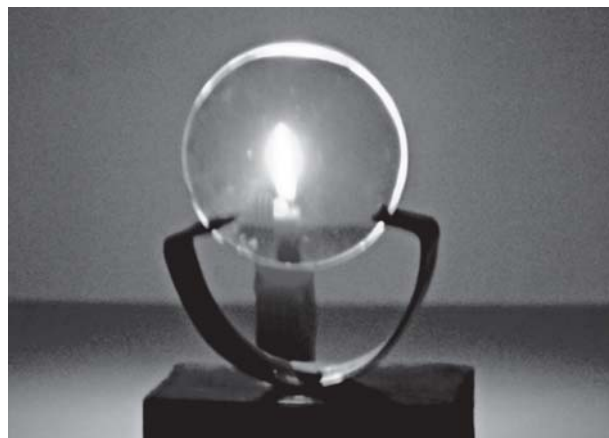
Fig. 15.27 Image formed by a concave lens
