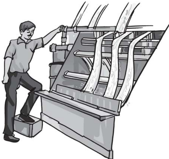
Fig. 3.8 (c) Scouring by machines
